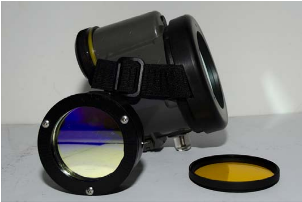
Nightsea Filters: BE3 Excitation Filter fitted to Inon Z240 (side view), BB62 Barrier Filter & Custom Sola Excitation Filter.
