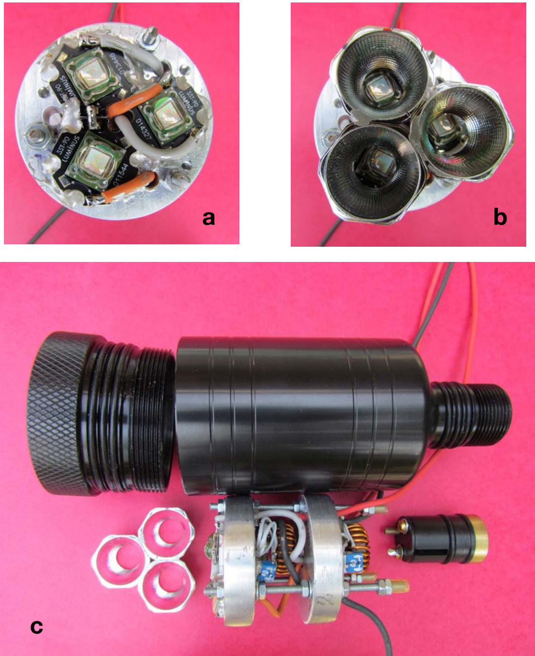
Fig. 18 HiTec Fluorescence with 3 blue LUMINUS LEDs
