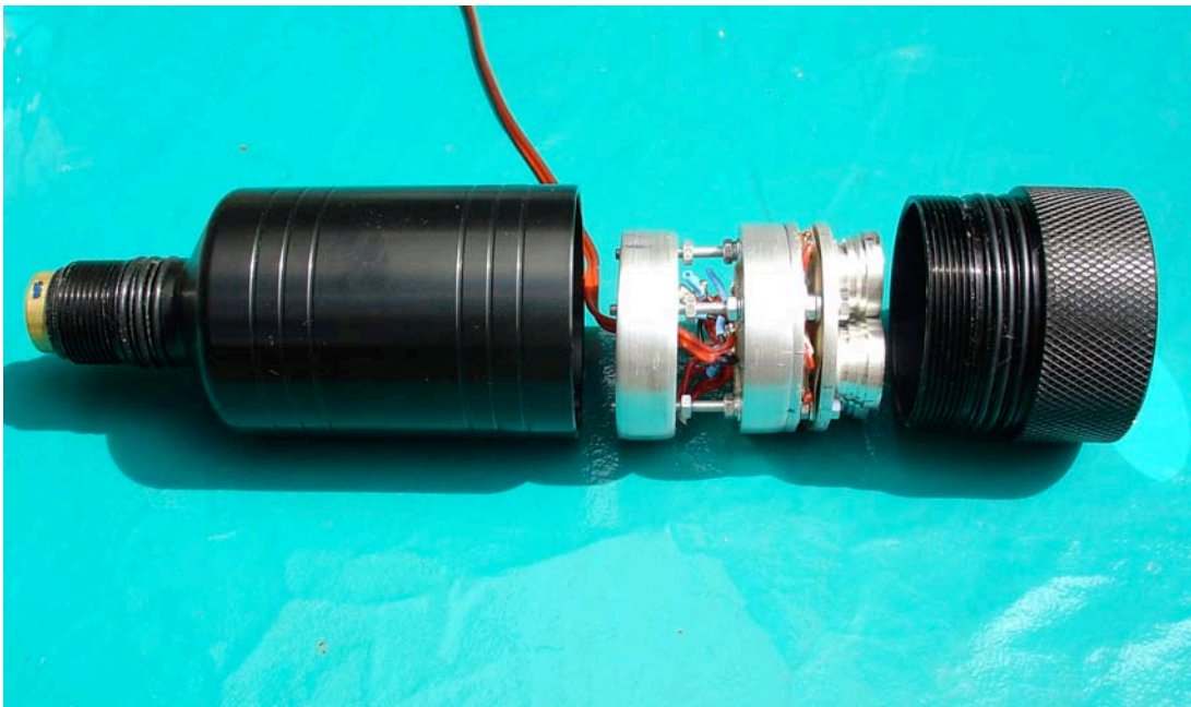
Fig. 17 Explosion diagram of the fluorescent torch. The black body was a former HID housing of TillyTec - Modular Power Lightsystem
