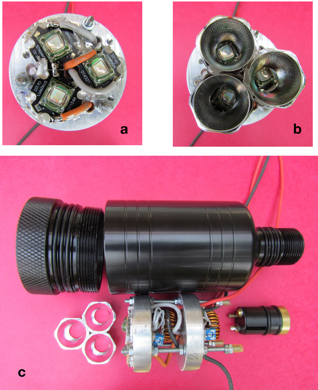
Fig. 18 HiTec Fluorescence with 3 blue LUMINUS LEDs
